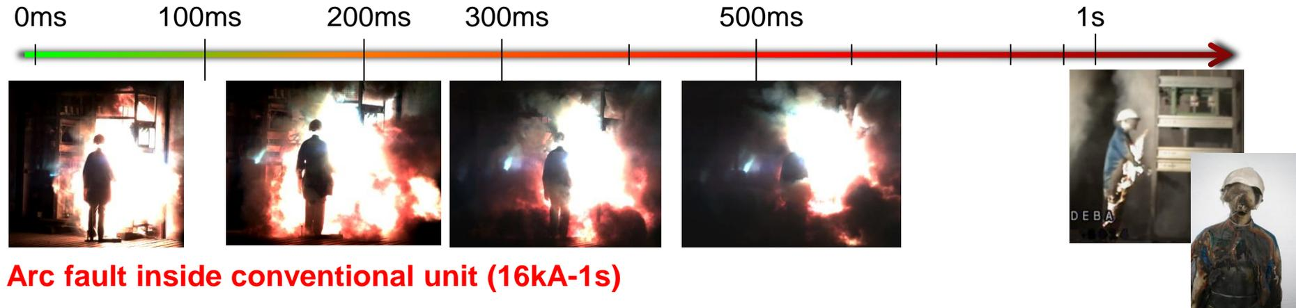
Arc fault inside conventional unit (16kA-1s)
